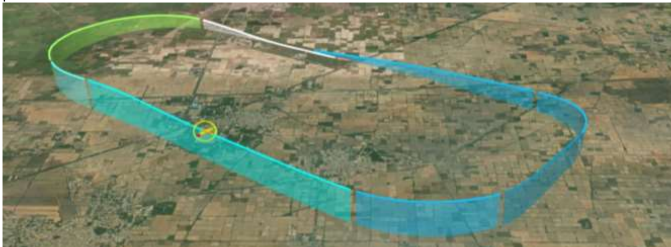
Figure 12: Circuit from runway 12 and final approach
